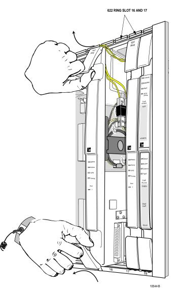
Figure 781-2. Example of Removing a Front Access Card
